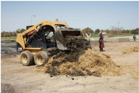
Figure 5: Pilling up dewatered sludge with straw 50:50
